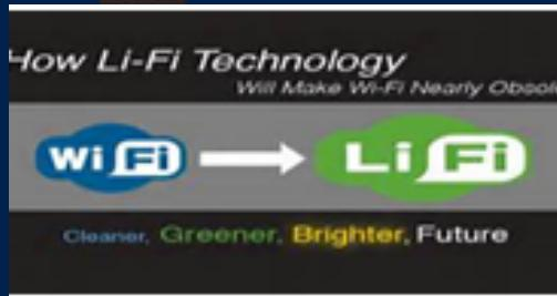
Li-Fi is a VLC, visible light communication technology, developed by the team of Scientists including professor Haas at the University of Edinburg and deals with Transfer of data through illumination by taking fiber out of optics by sending data .Through a LED light bulb that varies in the intensity faster than a human eye can Follow. Dr Haas amazed people by streaming
